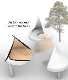
2. Roof cuts to see nature
